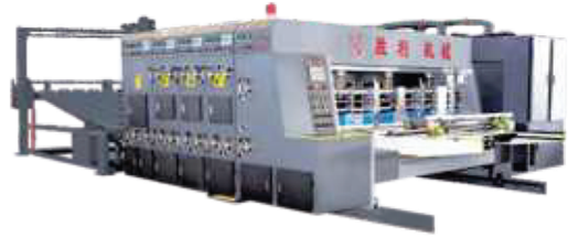
AUTOMATIC PRINTING, SLOTTING, CREASING, DIE CUTTING, STACKER WITH LEAD-EDGE FEEDER.
